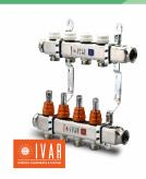
The 'manifold' is where each coil is connected to, and as each area is called on for heat, it distributes water at various flow rates which is determined by turning the orange flow metres accordingly.
