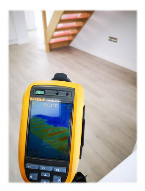
We use the latest in thermal imaging technology to give you the most precise indication of areas where existing UFH pipes are present. A fully trained Outsourced Energy technician will assist you with this service within the cost of hire.
