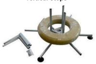
Place the pipe coil on the decoiler. Press the coil with the vertical stops and tighten the stops to the arms of the decoiler.
